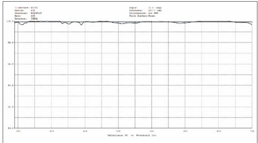
Figure 4. Optical Mirror - Reflectance vs. Wavelength Graph
