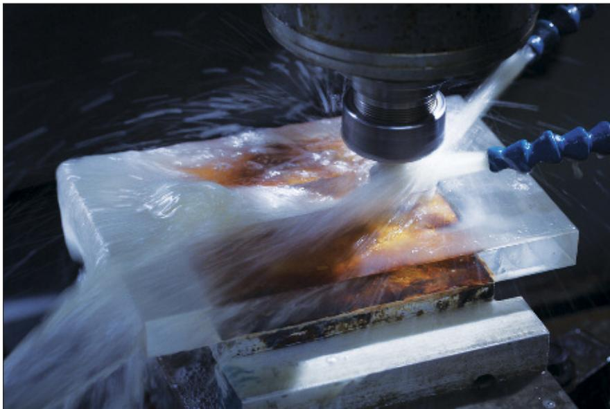
Figure 1. Machining was done on a Haas CNC machine using a custom-made fixture that held the part in place at  $12.5^\circ$ .
