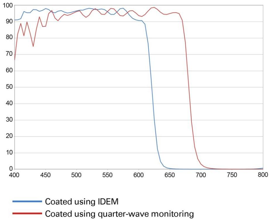
Figure 2 - The red line indicates optical monitoring with overshoots using quarter-wave monitoring; the blue line is the coating curve using the new IDEM monitoring system.
