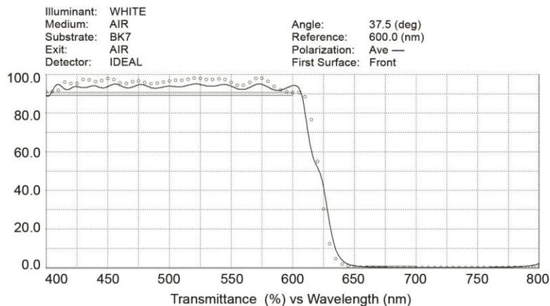
Figure 5 - The graph illustrates improved accuracy after the IDEM system was installed at PG&O. The original design curve is shown (black line), with the actual coating data imported, (represented by circles and superimposed over the design).
