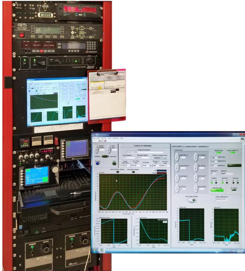
Figure 4 - SpectraLock Controller (left) and IDEM software screen capture (insert, right) during thin-film coating monitoring process.
