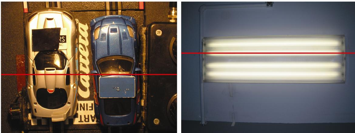
**Figure 2a (left):** Color photo of race cars with a red line showing where the line scan camera was focused.
