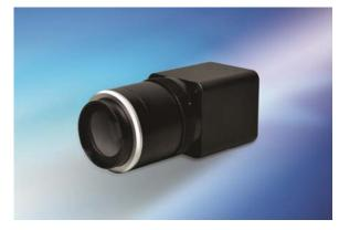
through atmospheric obscurants. It features 1280 x 720 pixels with 12.5 micron pitch and 30 frames per second (fps) at full frame rate. This next generation camera provides high-sensitivity in the SWIR spectrum ranging from 0.9 to 1.7 microns, with extended sensitivity into the NIR/SWIR spectral range from 0.7 to 1.7 microns. UTC Aerospace Systems is a unit of United Technologies Corp. (NYSE:UTX).
