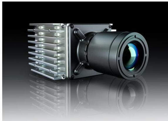
The rugged Vayu HD provides unprecedented image resolution utilizing a vanadium oxide microbolometer (VOx) sensor with a capacity of over 2.3 million pixels on a 12-micron pixel pitch, in a commercially-designed, IP67-environmentally rated, stand-alone camera. Other features include an athermalized 24 mm F1.1 custom-designed optic, 30 Hz frame rate, and three video formats: HD-SDI, h.264 IP-Video, or 16-bit Camera Link output. Custom lenses are available upon request.
