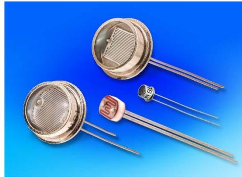
CdS photoresistors are ideal for street and solar lighting, audio compression and flame detection, camera light meters, and exposure and shutter controls applications. They can also be utilized in clock radios, alarm devices, outdoor clocks, and night light controls.
