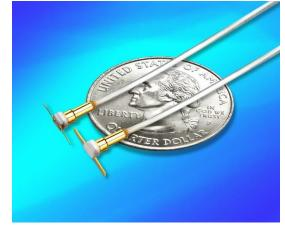
package pigtail assembly in solderable surface-mount configurations. For added convenience, the high-speed indium gallium arsenide PIN photodiodes are coupled directly to a single- or multi-mode pigtail fiber. The devices are also available with an internal fiber tip angle which is polished for low back reflection, and other customizable options.
