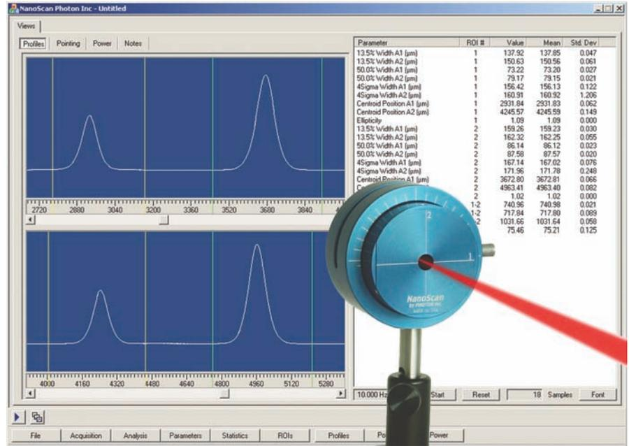
One large advantage in using a scanning slit profiler is that beams can be viewed directly with little or no power attenuation needed. Courtesy of Ophir-Spiricon.
