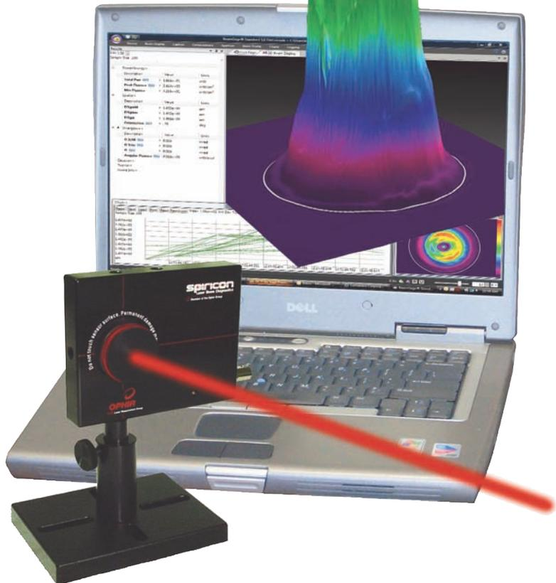
Camera-based systems capture the entire beam profile by using a CCD or CMOS camera, which provides a real-time 2- and 3-D image of the beam. Images courtesy of Ophir-Spiricon.
