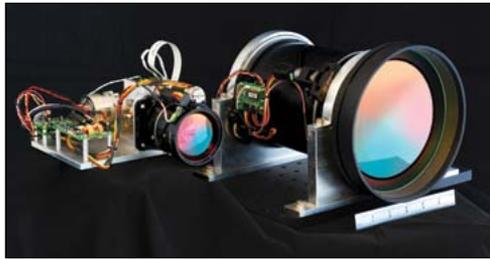
Figure 4: Sample test imagers representing the relative size and weight of MWIR (left) and LWIR (right) assemblies delivering  $<100 \mu\text{rad}$  IFOV performance necessary for quality ISR from typical, small UAVs.
