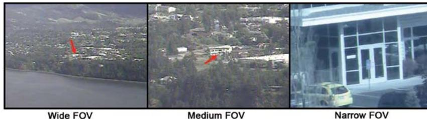
Figure 3: Current capability of advanced stabilized EO UAV payloads. Narrow field of view image represents standard definition (SD) imagery with a 0.30 degree HFOV. All images captured at 3,000 meters using Hood Technology's Alticam O9 EO.
