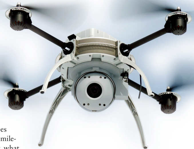
FIGURE 1. The Datron Scout (shown in flight) is an example of the 4.4 lb class of UAV for which public agencies may apply for an FAA Certificate of Authorization for use in the US National Airspace. (Courtesy of Datron World Communications)
