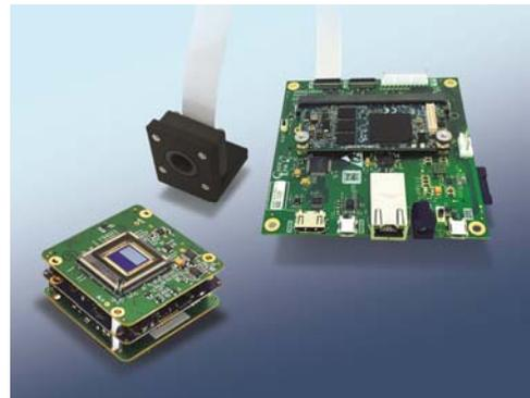
The company will demonstrate its latest **Embedded Vision Development Kit (VDK)** which integrates Basler's dart BCON camera with Critical Link's most popular processor board, interfaces, and onboard FPGA processing. In addition, Basler's Pylon camera software suite completes the kit's functionality. Visitors may enter to win an Embedded VDK, two of which will be raffled at the end of the show.
